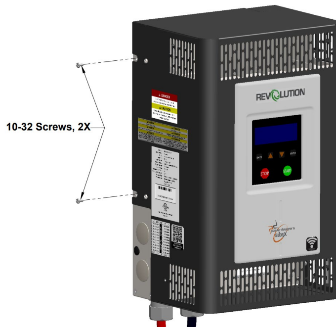
Figure 6: RVX05 Cover Removal
