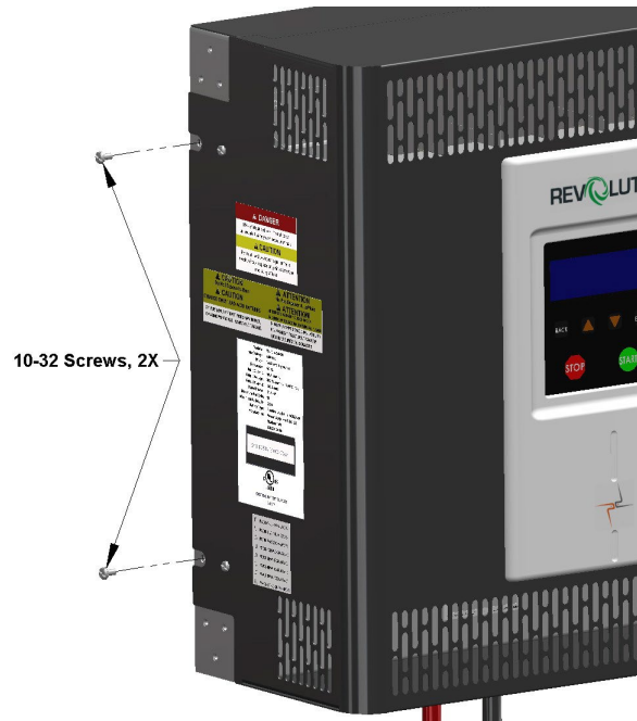
Figure 22: REX12 Cover Removal
